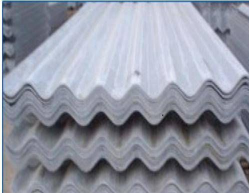
**Figure 1.** AC Roofing sheet stacked
