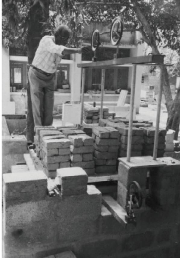
**Figure 6.** Static uplift load tests on roofing sheets
